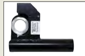
'Dust Director' tuck pointing guard Accepts 4", 4/12", 5" and 6" diameter diamond blades. Port is 2". Not for use with Type 1 or Type 27 bonded abrasives.
